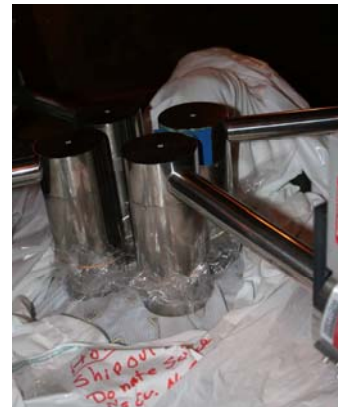
Four thin planar germanium detectors positioned over the chest to measure ^{241}\text{Am} activity in the lungs of Case 0407.
